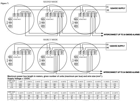
For 24VDC supply voltage, the maximum power bus length is 4 times as long as 12VDC supply voltage. Maximum interconnect bus length: 2000 meters, 0.75mm<sup>2</sup> or larger cable. All wiring must conform to local electrical codes.
