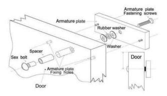
Armature plates must be fixed as shown above. Do not over tighten the fixing screw. The armature must be allowed to 'float' on the rubber washer.
