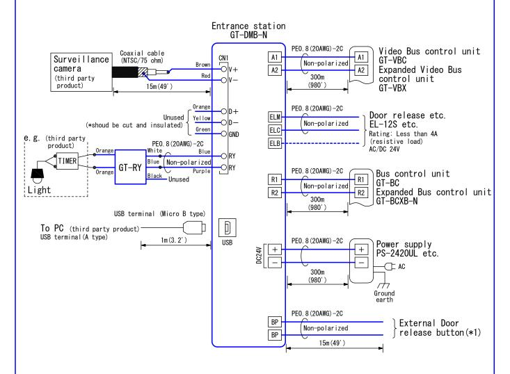
PE: Polyethylene-insulated PVC jacket cable
