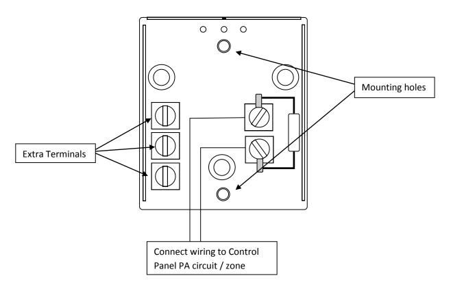
Note: Three extra terminals are provided for terminating other circuit wires.
