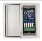
PCR43305RE 5-Channel Receiver enclosed in an IP66 case
