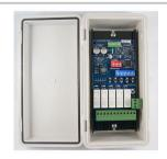
PCR43305RE 5-Channel Receiver enclosed in an IP66 case
