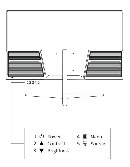
**KEY FUNCTIONS** (located under the lower right-hand edge of the monitor)
