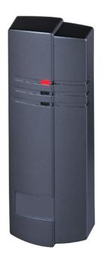
The SMART6000 Mifare Reader is available as a 26/34/40 bit CNS reader and can also be provided as customer-secured sector reader if required, with standard 26/32/34 bit wiegand output.
